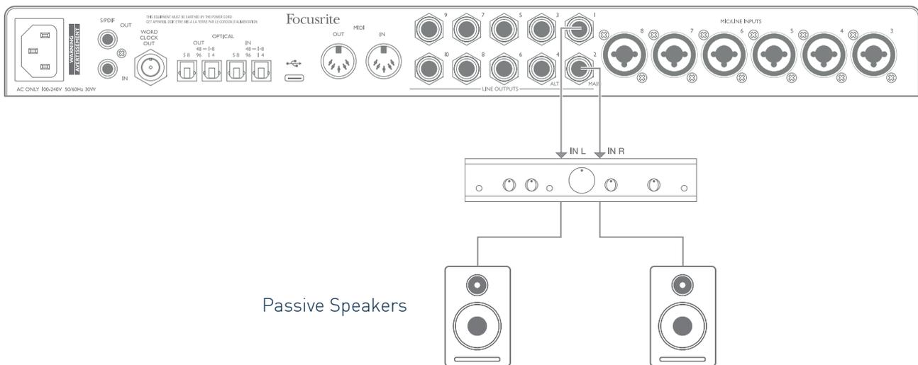
All the line output connectors are 3-pole (TRS) 1/4" (6.35 mm) jack sockets, and are electronically balanced. Typical consumer (hi-fi) amplifiers and small powered monitors will probably have unbalanced inputs, either on phono (RCA) sockets, or via a 3.5 mm 3-pole jack plug intended for direct connection to a computer. In either case, use a suitable connecting cable with jack plugs at one end.
