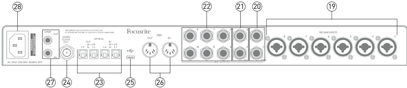
19. **MIC/LINE INPUTS 3 to 8** – Combo type input sockets - connect further microphones or line level signals via XLR or ¼” (6.35 mm) jacks as appropriate. Either ¼” TRS (balanced) or TS (unbalanced) jack plugs can be used for line level signals.
