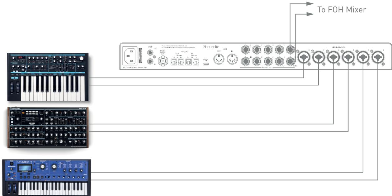
In the example illustrated, three stereo keyboards are connected to the rear panel inputs of the Scarlett 18i20; Outputs 3 and 4 go to the main PA system. The performer can adjust the gain for the individual keyboards from the front panel; he/she can also adjust the overall level of the keyboard mix.
