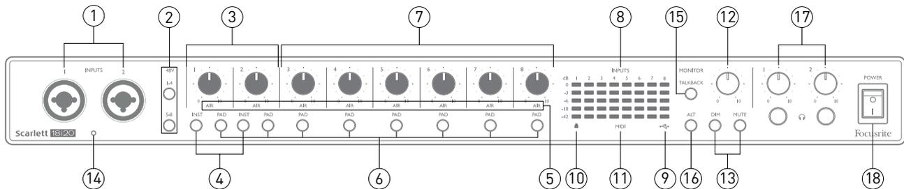
The front panel includes all the input gain and monitoring controls as well as two of the input connectors for Mic, Line and Instrument signals.
