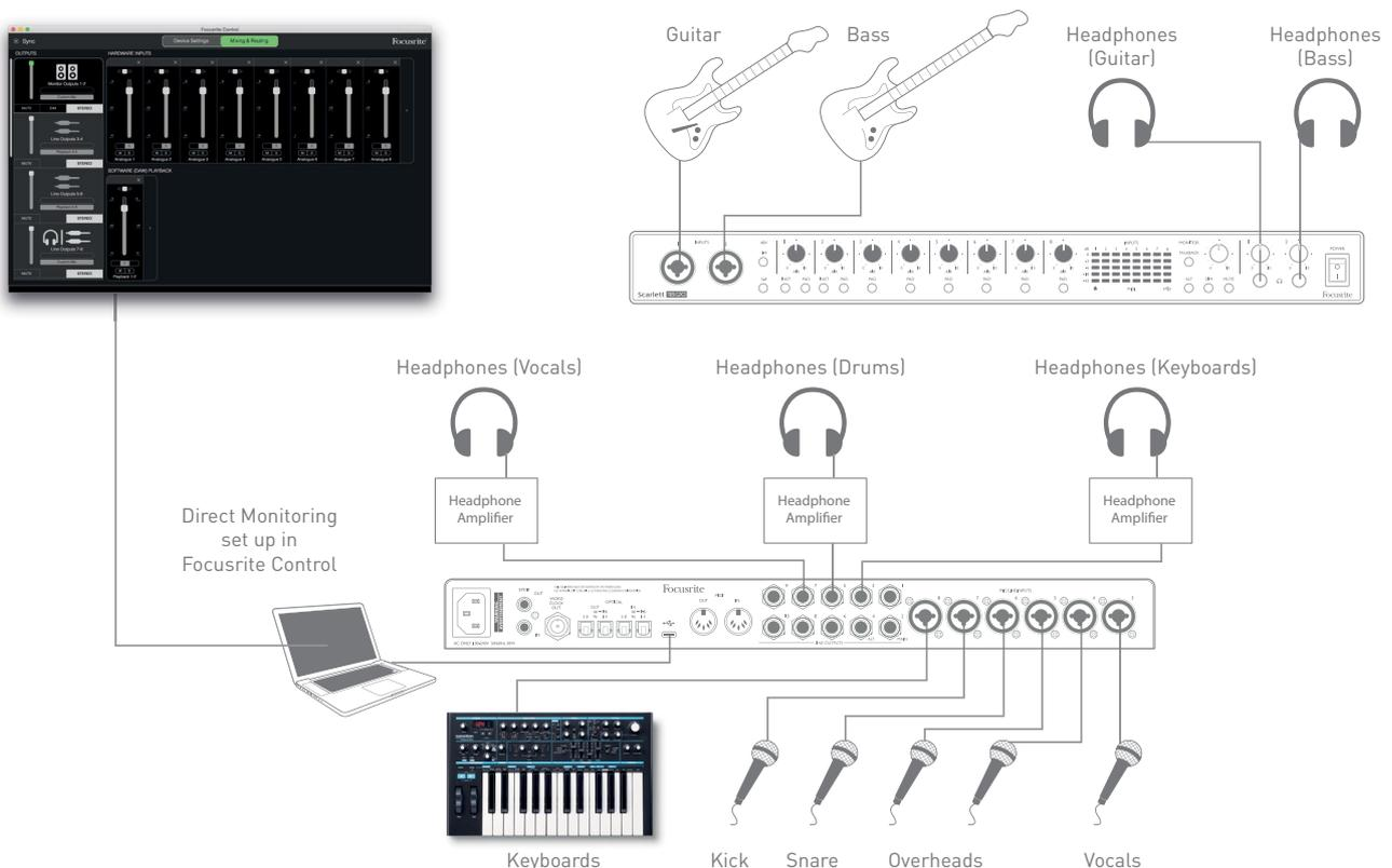
When using Direct Monitoring, ensure your DAW software is not set to route any inputs (what you are currently recording) to any outputs. If it is, the musicians will hear themselves “twice”, with one signal audibly delayed as an echo.
