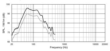
Frequency response (1W, 1 m) is measured on-axis with two boundary junction (pi loading, gray line) and with three-boundary junction (pi/2 loading, black line)
