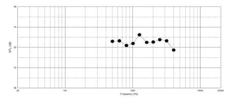
Contribution of each mid-range one-third-octave frequency band to the SPL (per EN54-24) when system is driven to Rated Maximum SPL (92 dB @ 4m; 101 dB @ 1m) using specified broadband pink-noise signal, 60W tap setting, 4m (Contribution figures: 500 Hz = 78.16 dB; 630 Hz = 78.59 dB; 800 Hz = 76.65 dB; 1000 Hz = 77.97 dB; 1250 Hz = 82.76 dB; 1600 Hz = 79.41 dB; 2000 Hz = 80.48 dB; 2500 Hz = 82.88 dB; 3150 Hz = 81.62 dB; 4000 Hz = 76.67 dB).
